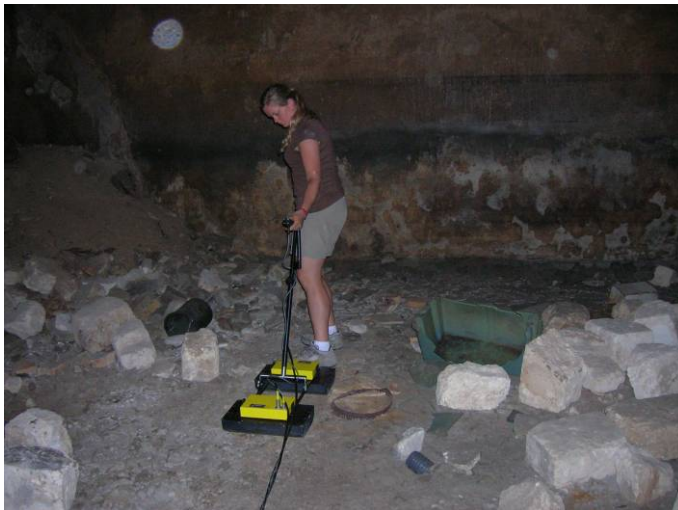
Figure 9: Left: Data being collected with 225 MHz antennae within a cistern behind the Cactus House. Right: GPR profile (225 MHz) collected along the rubble laden floor of the cistern.
